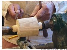
Now mark the cylinder at the midpoint, quarter and eighth points with a pencil, and using a fingernail gouge start to shape the ball, working from the outside markers first, and then moving in.
