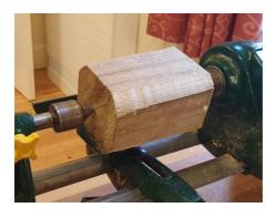
The aim was to make a 90mm diameter ball. Start with a block of wood slightly wider than 90mm and long enough to leave a spigot on each end.
