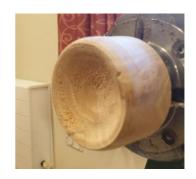
Roy then showed us his method, which uses a similar marking system with the pencil, but he cuts 45° flat angles, working progressively in from the outside, and then finishes off by eye.
