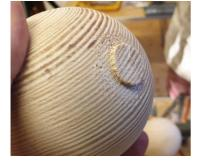
The pegs can be parted off with a saw. To clean up the ends the ball must be mounted between pre-prepared cup shaped holders.
